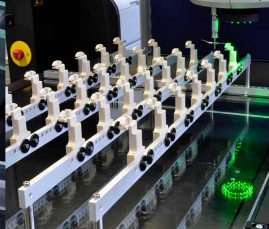
Image above: Measuring a component for the semiconductor industry using a laser sensor.
